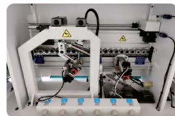
Corner Trimming unit to round the 4 corners is equipped with 2 HF motors, to get a smoother corner effect, usually work for 2mm thickness edging tape.
