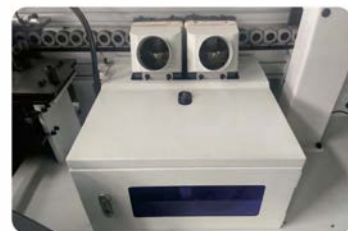
There are two counter rotating shaper cutters there are independent control of air cylinders allows milling of front edge and back edge without tear out.
