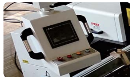
Control panel: Touch screen control panel, Taiwan Delta brand control system
