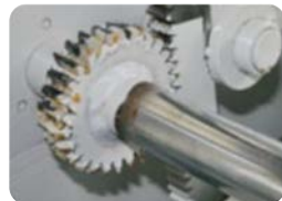
Rack And Pinion For Flatness Control
