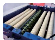
Feeding Rollers 6 Groups/12 Pieces. Very strong to press and feed smoothly.
