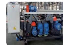
Individual motor to each spindle to ensure maxim cutting.
